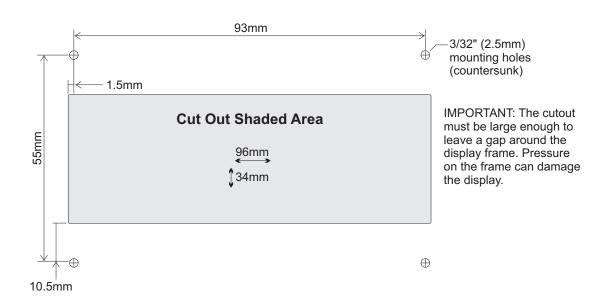
You may use this drawing as a template: Tape it over the mounting location and drill/cut directly through the paper. If you use this method, make sure to **measure the printed drawing** carefully and adjust printer settings if needed to ensure that the drawing is printed exactly to the correct dimensions both horizontally and vertically.
